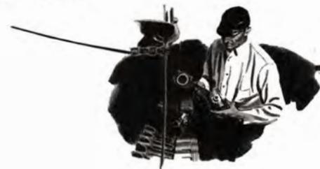
Pistons checked for perfect contour and profile. Then measured in controlled-temperature test rooms. Held to weight limits of 39 ten-thousandths of a pound.
