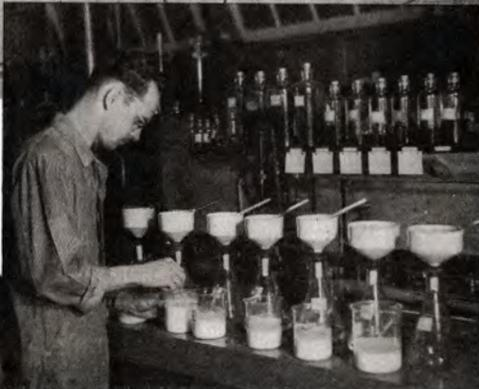
Motor oils get "tired," just as you do, after working for a long stretch. Oxidation-acids are formed. Here a Pennsylvania laboratory worker filters out these "fatigue" acids for special study and analysis. This is one of many researches at State College, Pennsylvania, helping to keep emblem-protected Pennsylvania Motor Oils so far ahead in lasting quality, and lubricating value, in your car.
